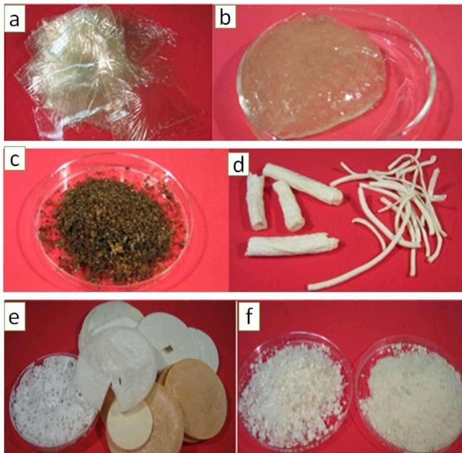
Figure 1.14 Different forms of Chitosan for biomedical applications (a) films, (b) gels, (c) microspheres, (d) tubes, (e) sponges and (f) powder (67).
